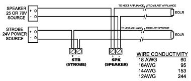
\* MAX. WIRE DISTANCE (IN FEET) =  $\frac{\text{PANEL VOLTAGE - DEVICE MINIMUM VOLTAGE}}{\text{TOTAL CURRENT DRAW}} \times \text{WIRE CONDUCTIVITY (STROBE ONLY)}$
