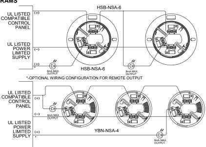
NOTE: Fire alarm control panel compatibility is required for DCP products. DCP communications protocol allows system components (DCP sensors AIE-EA, ALG-V, ALO-V, ACA-V, ACC-V, ALK-V, ALN-V, ATJ-EA and ATG-EA, bases and modules)
