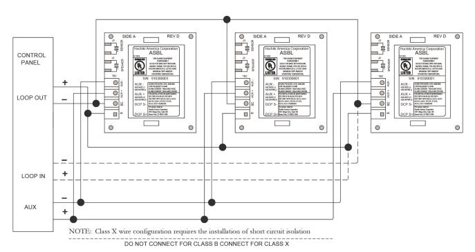
NOTE: Fire alarm control panel compatibility is required for DCP products. DCP communications protocol allows system components (DCP sensors AIE-EA, ALG-V, ACA-V, ACC-V, ALK-V, ALN-V, ATJ-EA, ATG-EA, ALO-V ACD-V, bases and modules) to be used concurrently on a system's SLC (Signaling Line Circuit).
