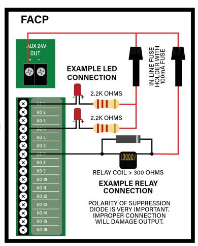
Outputs are intended to be connected to a 24VDC load. The other side of this load should be connected to a 24V power source, such as the panel's AUX24V+ terminal.
